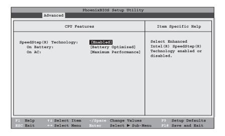
Figure 8. CPU Features Submenu
